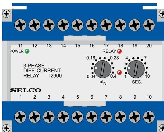
The output relay is a latching relay. The latching can be reset or disabled by bridging terminals 5 and 6.
